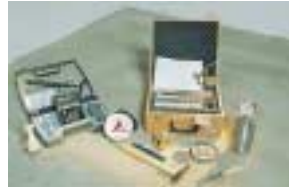
Testing the moisture content of the substrate and checking temperature and relative humidity in the room.
